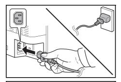
4 Connect one end of the supplied power cable to the machine and the other end to a power outlet.
